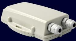
Robust battery-powered or wired GPS tracking device with inputs/outputs, I<sup>2</sup>C Sensor Interface, and WiFi Positioning for indoor and outdoor asset tracking and sensor monitoring
